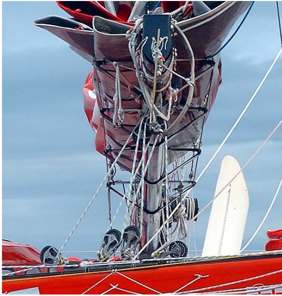
Figure 10: Healthy sheave to line ratio on maxi trimaran IDEC. Photo: J. Paul Riou.
